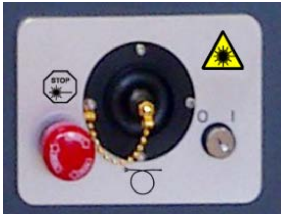
front panel labeling
