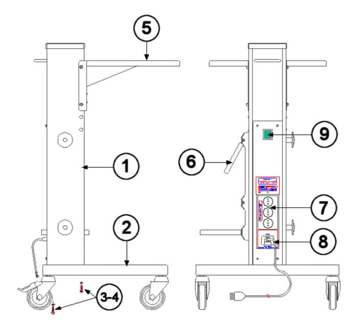
a. Assemble the cart column (1) on the base with wheels (2) using the screws (3) and the washers (4) and the supplied Allen wrench.
